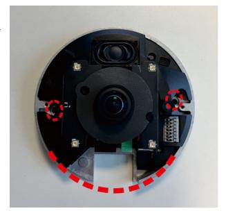
On the ceiling or wall, draw a dot 20 mm above the center of the marked concave edge.
