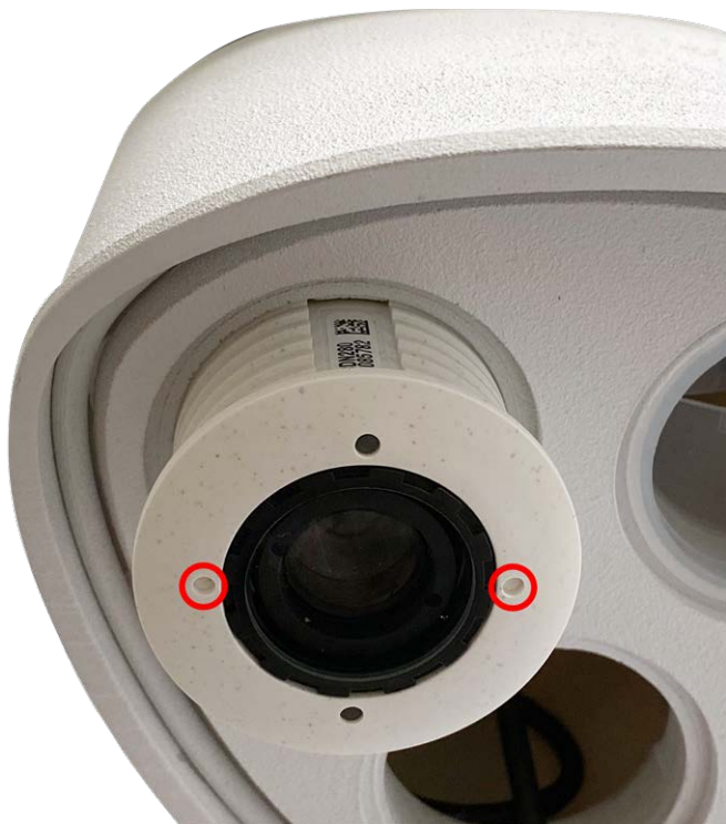
Fig. 13: Insert sensor module into module housing
