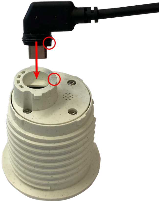
Fig. 28: Connect the sensor module cable
