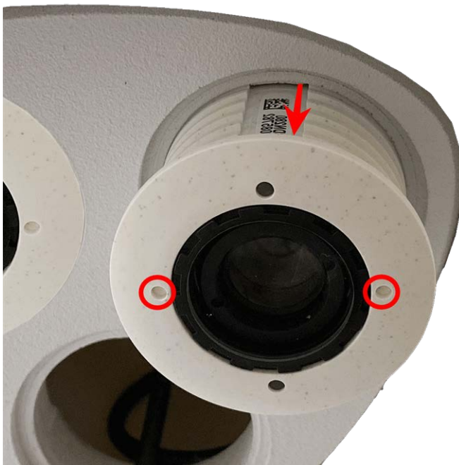
Fig. 24: Remove sensor module from the module housing
