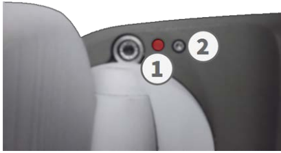
Fig. 75: View of the MOBOTIX M73 from below with LED ① and screw with sealing ② that hides the key inside the camera body
