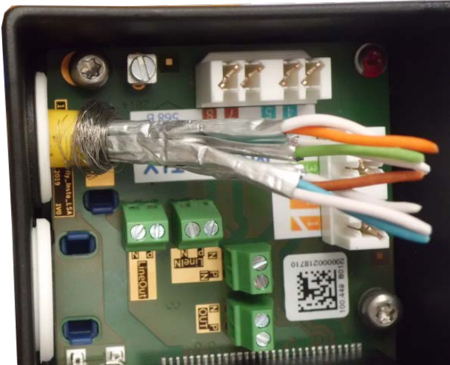
Fig. 57: Network cable inserted, plug properly seated
