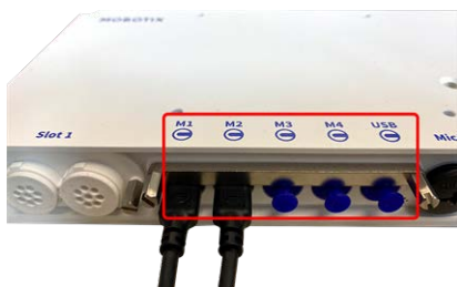
Fig. 37: 4 Module Connector Ports and 1 USB-C interface
