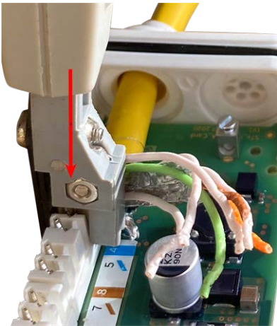
Fig. 25: Network wires connected using LSA+/Krone tool
