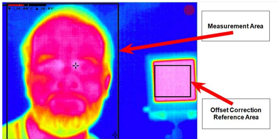
Fig. 18: Live screen after defining the Measurement Area and the Offset Correction Reference Area
