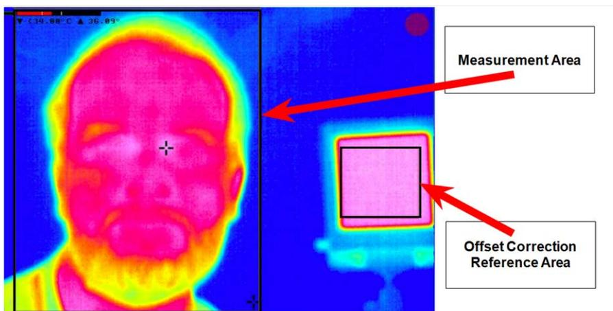
Fig. 1: Live image with *Measurement Area* and *Offset Correction Reference Area* (black body)
