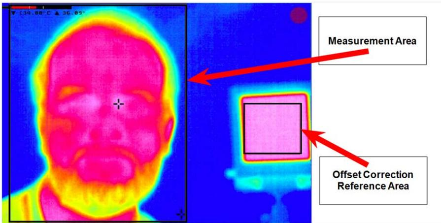
Fig. 5: Live image with Measurement Area and Offset Correction Reference Area (black body)
