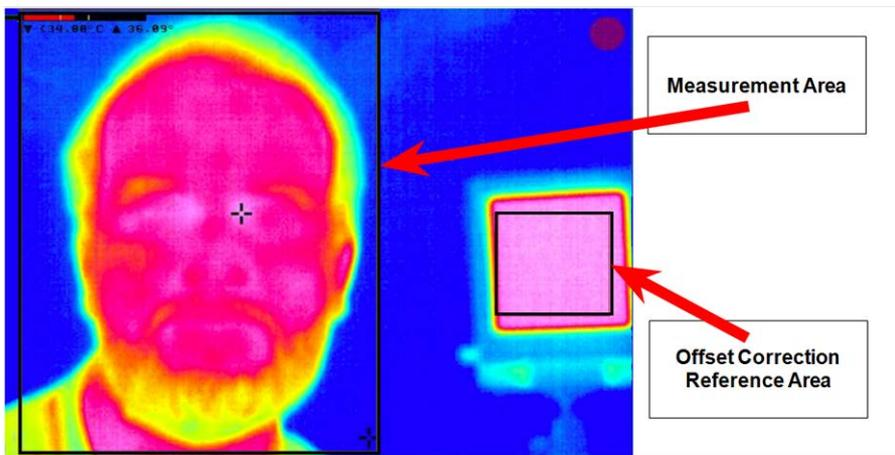
Fig. 25: Live image with Measurement Area and Offset Correction Reference Area (black body)
