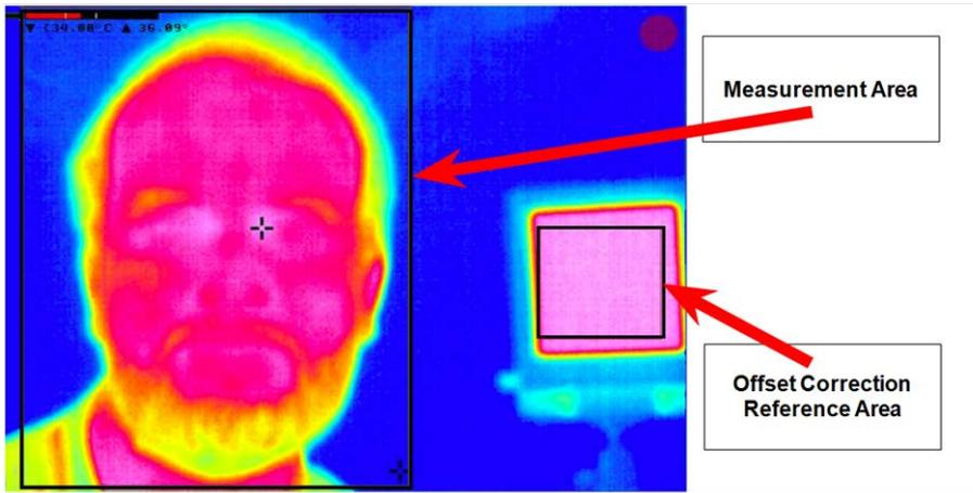
Fig. 21: Live image with *Measurement Area* and *Offset Correction Reference Area* (black body)
