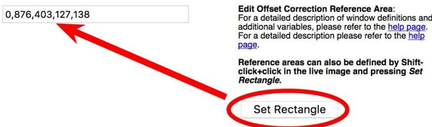
Fig. 16: Setting the offset correction reference area
