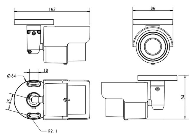
Fig. 1: 2MP Bullet Camera: All measurements in mm
