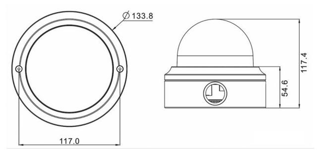
Fig. 1: 2MP Vandal Fixed Dome Analytics Camera: All measurements in mm
