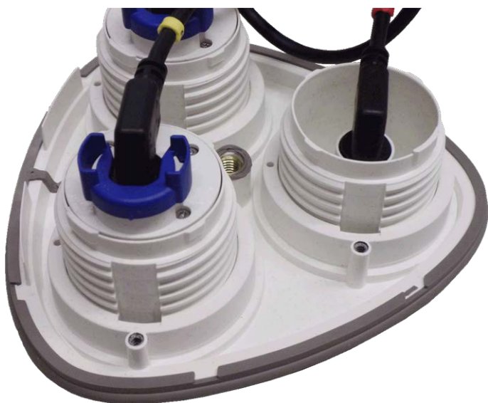
Fig. 16: Default front plate with sensor modules (back)
