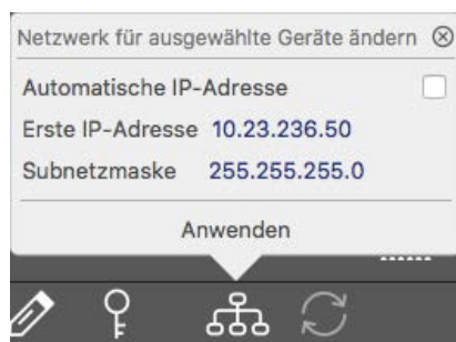
Fig. 82: Change network settings for selected devices
