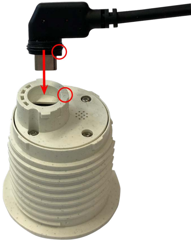
Fig. 10: Connect the sensor module cable
