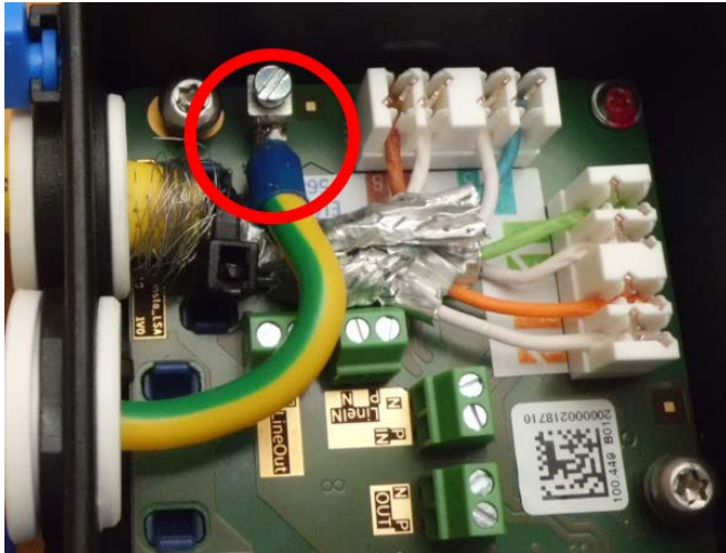
Fig. 63: Ground wire connected to terminal
