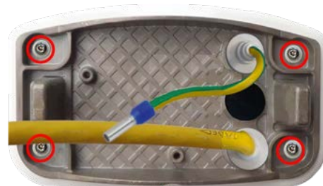
Fig. 51: Installed and ready for Connector Box LSA
