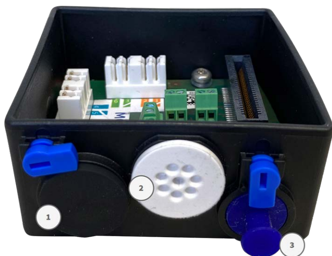
Fig. 53: Connector Box LSA with rubber plug black C.3 ① , rubber plug single-wire C.4 ② , USB plug ③ and two blue locks
