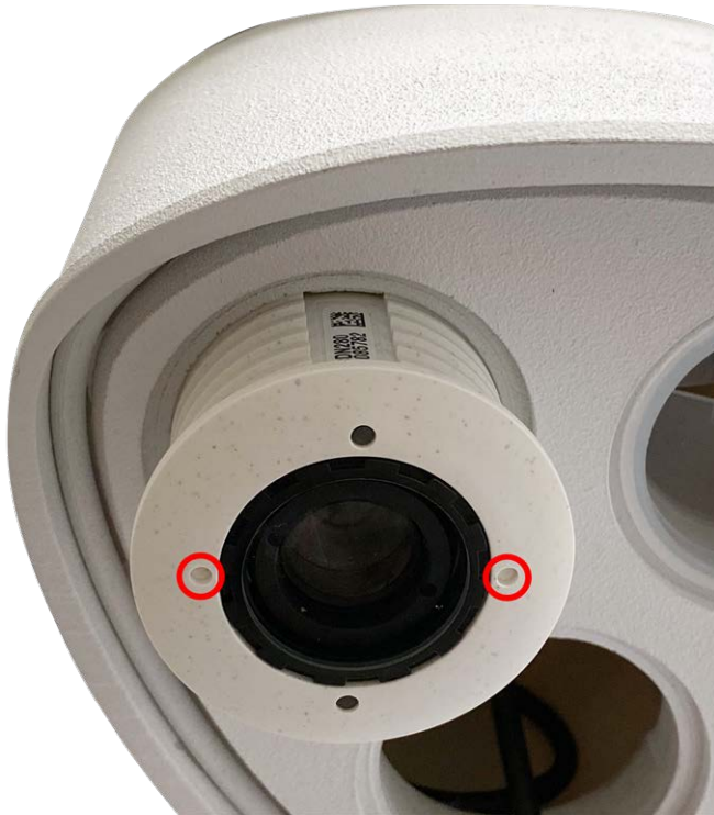
Fig. 23: Unlock the sensor module
