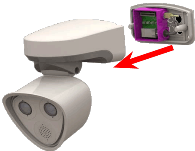
Fig. 94: Pull the camera body off the mounting plate
