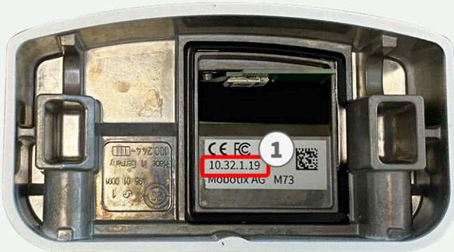
Fig. 6: IP address on the back of the camera housing
