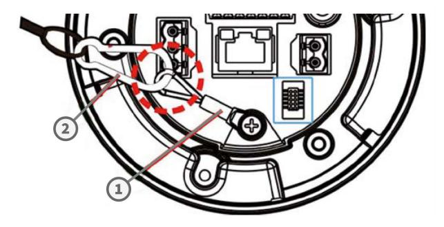
**NOTE!** For safety reasons, it is recommended to hook up the camera's anti-drop ring ① with the anti-drop chain ② of the pendant when installing the camera. For more information about the pendant and anti-drop chain, please see the corresponding Quick Installation document available at www.mobotix.com > Support > Download Center > Marketing & Documentation > Manuals in the *Speed Dome Accessories* section..
