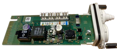
Fig. 19: S74 Network Slide in Board with LSA terminal
