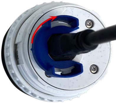
Fig. 11: Lock sensor module cable
