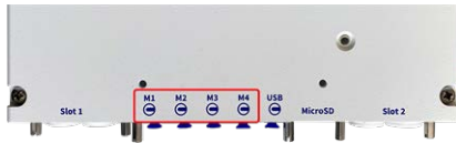
Fig. 38: Module connectors of the MOBOTIX S74
