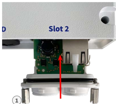
Fig. 18: Connecting the S74 Network Slide in Board with RJ45 socket
