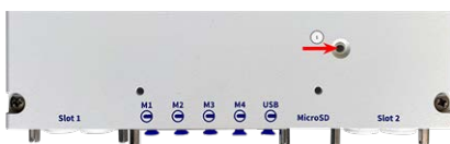
Fig. 41: Camera LED on top of the camera body
