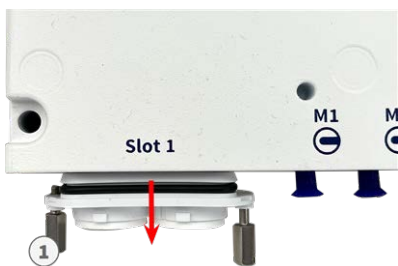
Fig. 31: Remove cover from interface board slot
