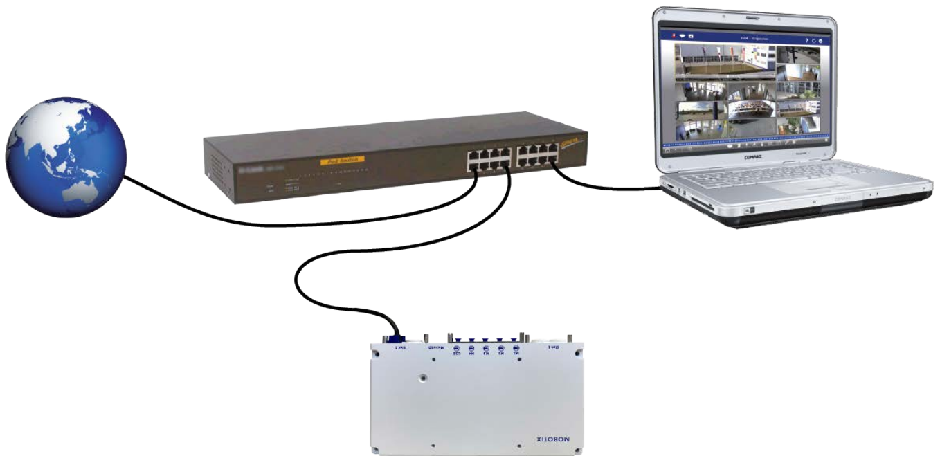
Fig. 39: Power supply using PoE switch according to PoE Plus (802.3at-2009)
