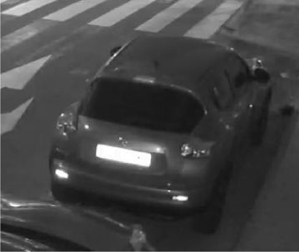
Fig. 17: Over exposed license plates due to too strong IR LED light
