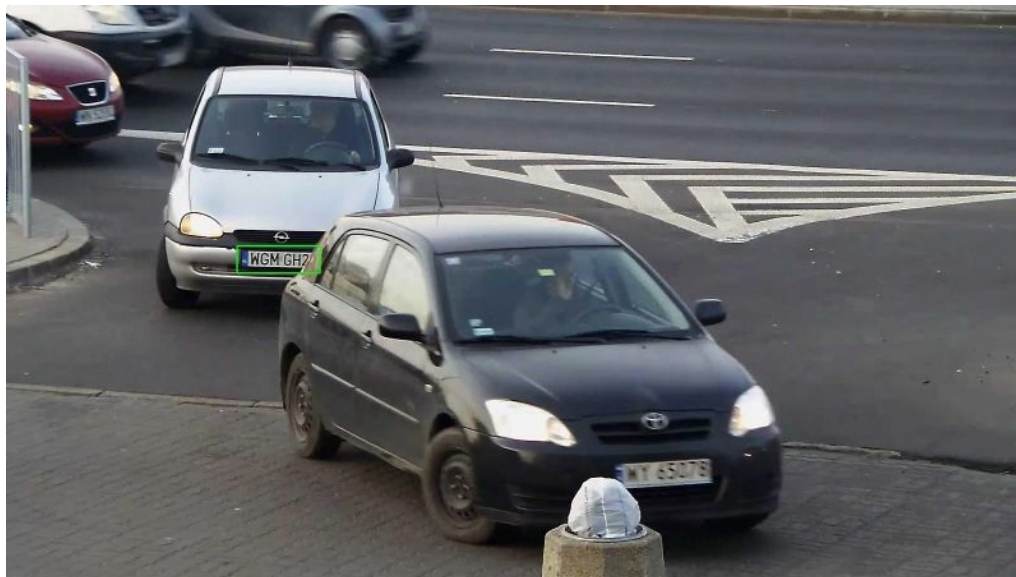
Fig. 12: Insufficient depth of field
