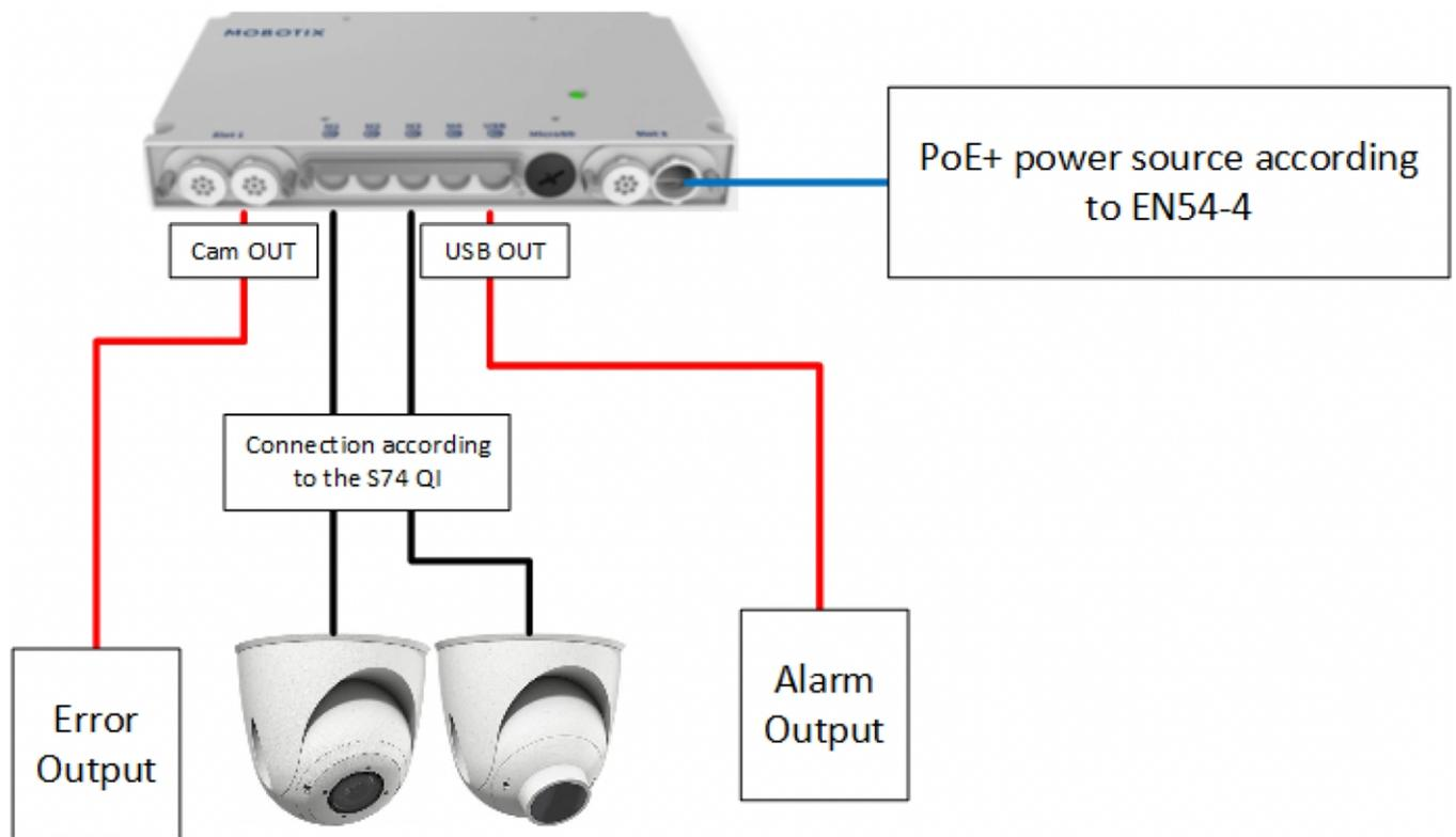
Fig. 2: Installation compatible CNPP du MOBOTIX S74
