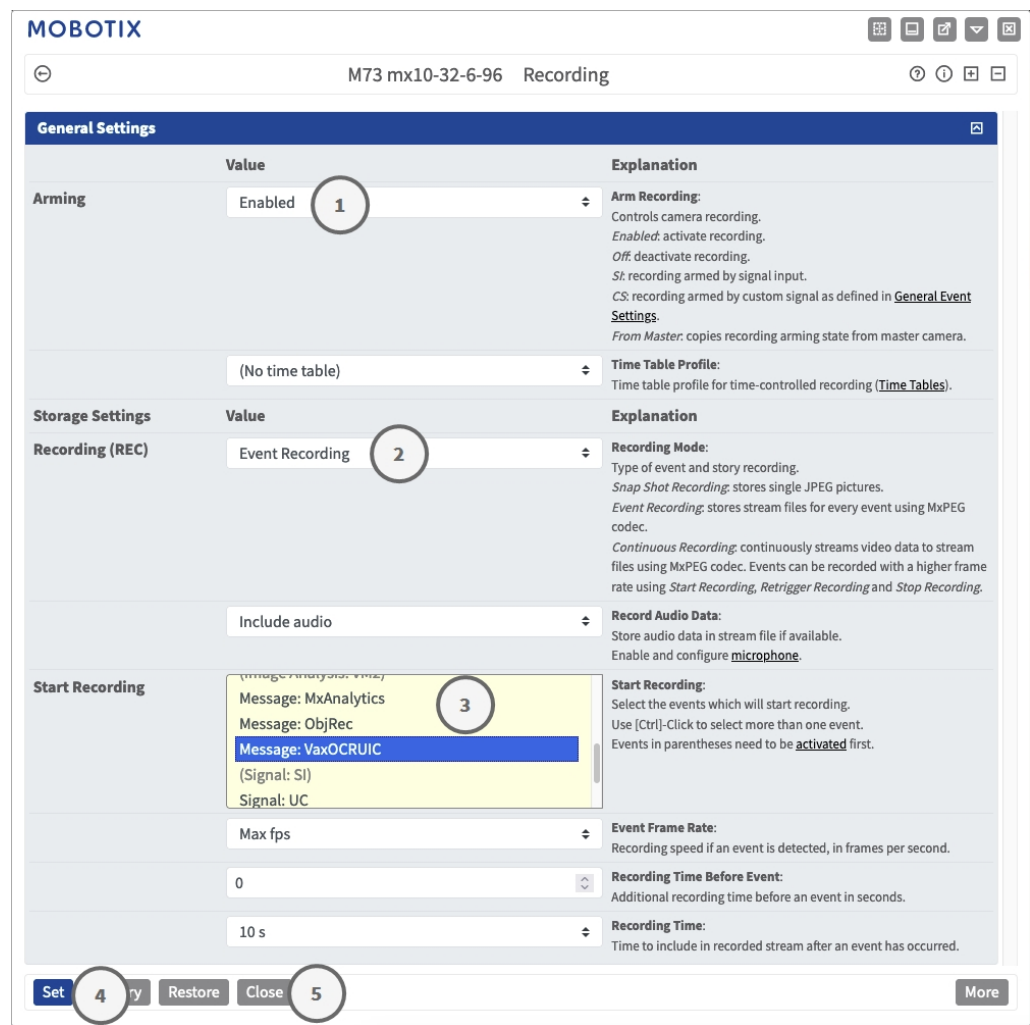
Fig. 24: Configuration of camera recording settings
