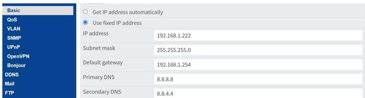
The screenshot shows the configuration interface for a MOBOTIX camera. On the left is a dark blue sidebar menu with the following items: Basic, QoS, VLAN, SNMP, UPnP, OpenVPN, Bonjour, DDNS, Mail, and FTP. The 'Basic' menu item is highlighted. The main content area is a light gray form with the following settings:
