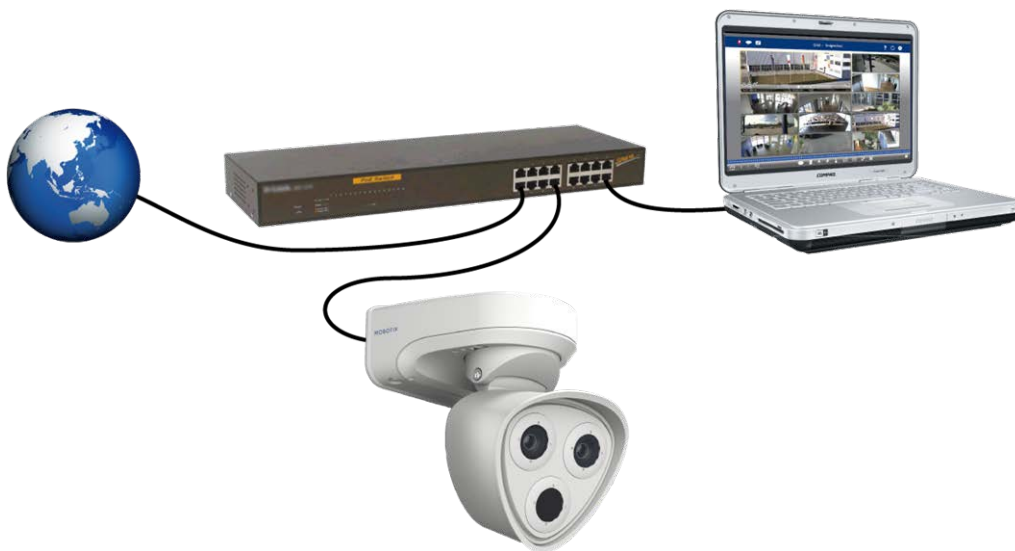
Fig. 26: Power supply using PoE switch according to PoE Plus (802.3at-2009).
