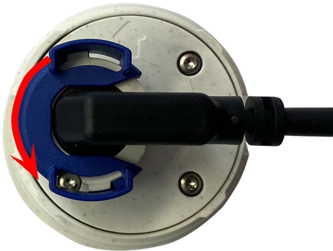
Fig. 15: Unlock sensor module cable
