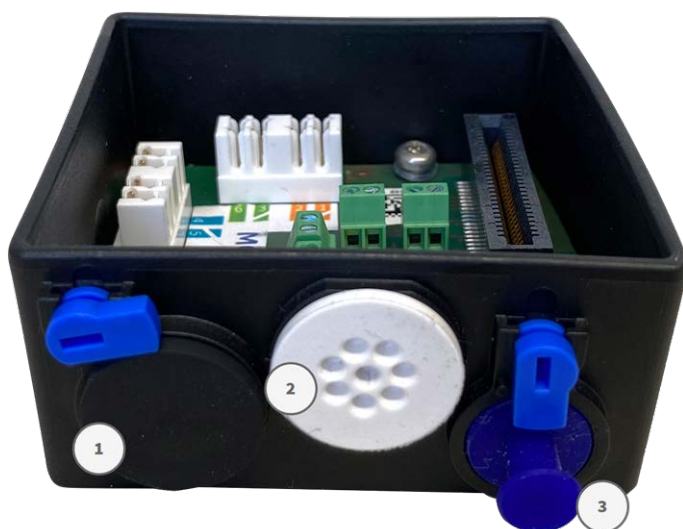
Fig. 27: Connector Box LSA with rubber plug black C.3 ① , rubber plug single-wire C.4 ② , USB plug ③ and two blue locks
