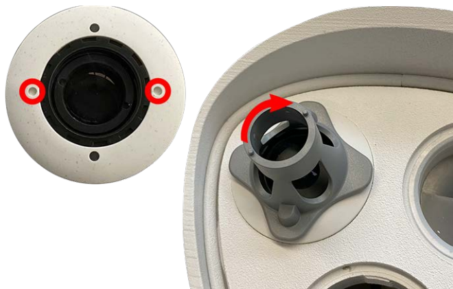
Fig. 12: Lock the sensor module
