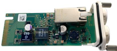
Abb. 16: S74 Network Slide in Board with RJ45 socket
