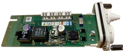
Abb. 19: S74 Network Slide in Board with LSA terminal
