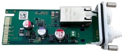
Abb. 29: S74 Network Slide in Board with RJ45 and VDC power supply
