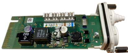
Fig. 19: S74 Network Slide in Board with LSA terminal
