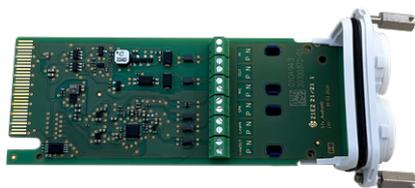
Fig. 30: S74 IO Slide in Board
