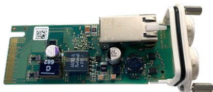
Fig. 16: S74 Network Slide in Board with RJ45 socket
