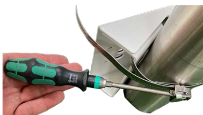
Fig. 14: Tighten the straps
