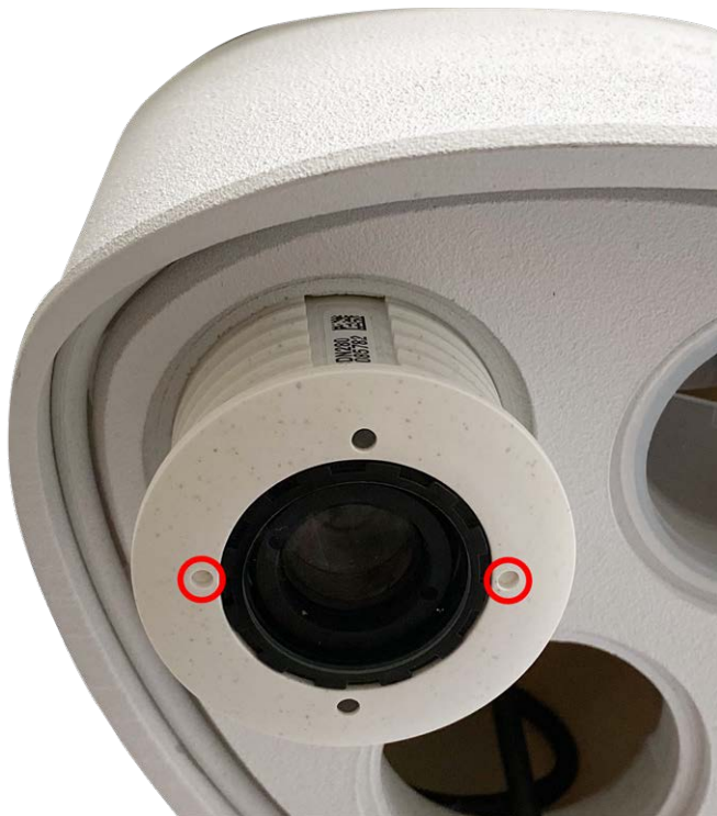
Fig. 11: Insert sensor module into module housing
