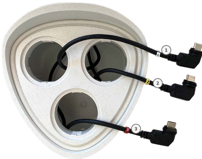
Fig. 8: Numbered sensor module cables
