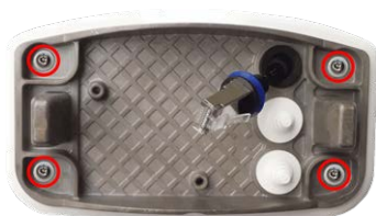
Fig. 18: Installed and ready for Connector Box RJ45
