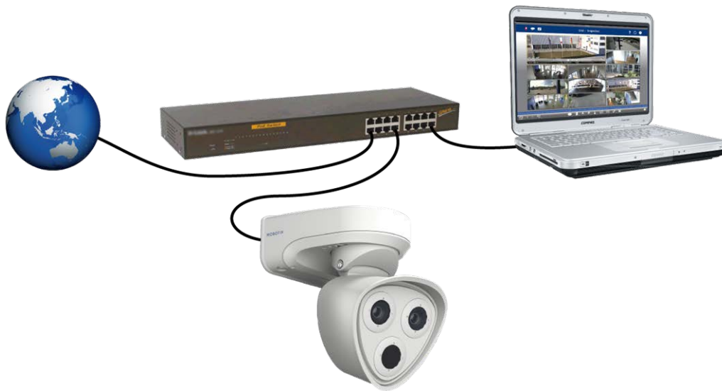
Fig. 25: Power supply using PoE switch according to PoE Plus (802.3at-2009).
