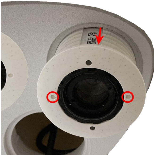
Fig. 17: Remove sensor module from the module housing
