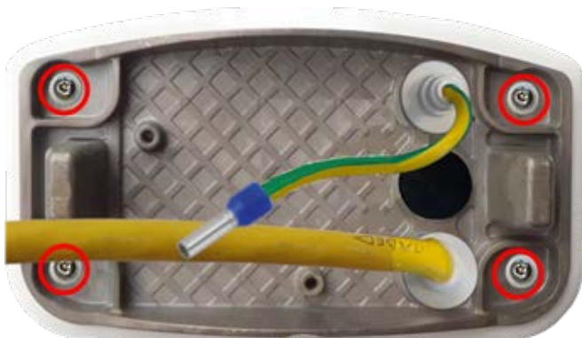
Fig. 28: Mounting plate with ground wire and network cable
