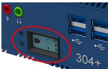
Press the Up/Down buttons to the left of the display to switch between these display modes:
