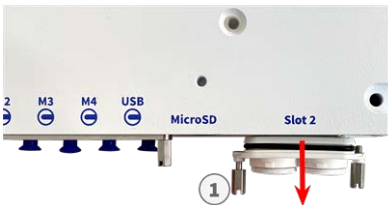
Fig. 12: Remove cover from interface board slot
