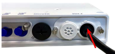
Fig. 29: Press the plug in firmly until the blue sealing ring clicks into place
