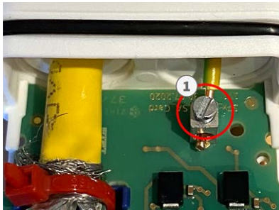
Fig. 18: Ground wire connected to terminal
