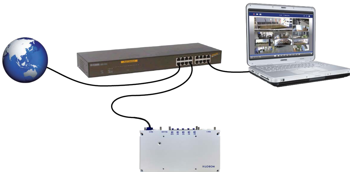
Fig. 28: Power supply using PoE switch according to PoE Plus (802.3at-2009)
