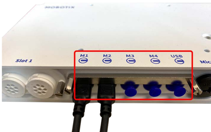
Fig. 26: 4 Module Connector Ports and 1 USB-C interface
