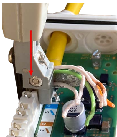
Fig. 16: Network wires connected using LSA+/Krone tool
