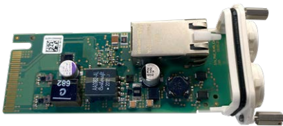
Fig. 7: S74 Network Slide in Board with RJ45 socket
