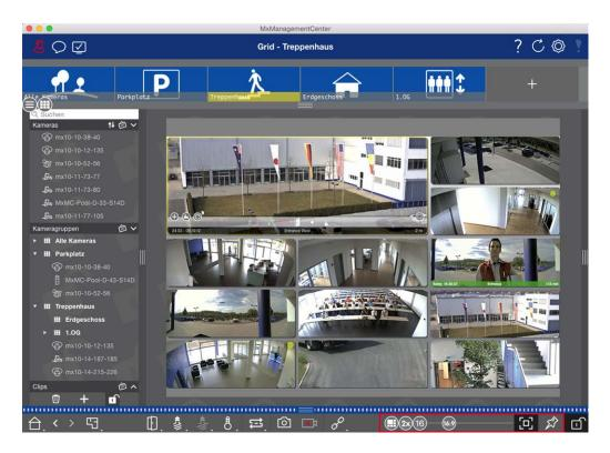
Fig. 45: Setting the layout for the Grid View
