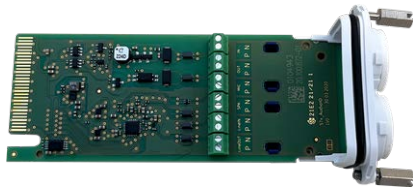
Fig. 17: S74 IO Slide in Board
