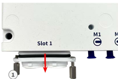
Fig. 18: Remove cover from interface board slot
