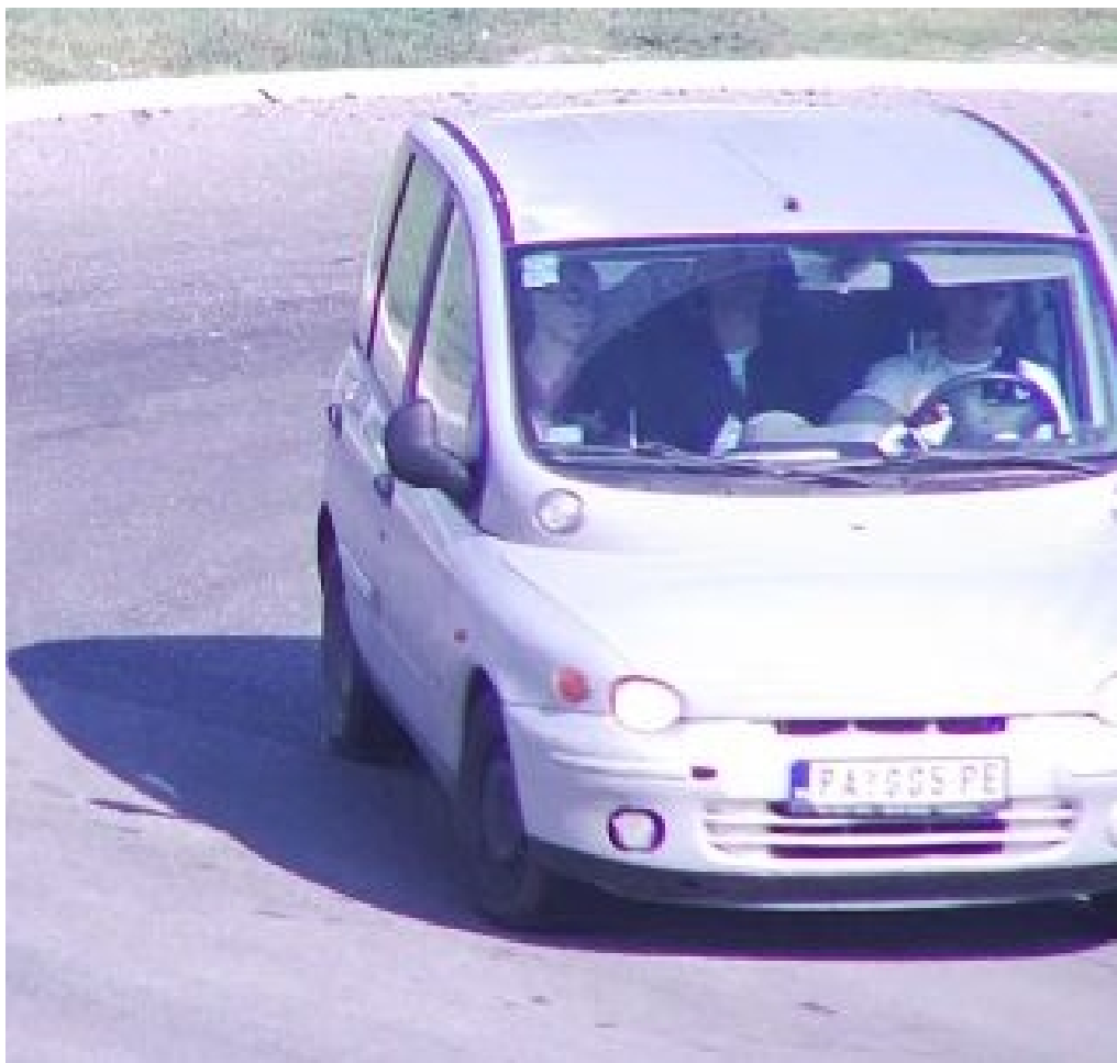
Fig. 16: Over exposed license plate at daytime
