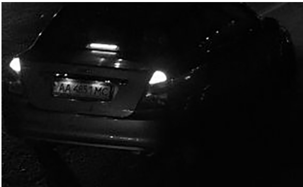
Fig. 18: Insufficient light to recognize license plate
