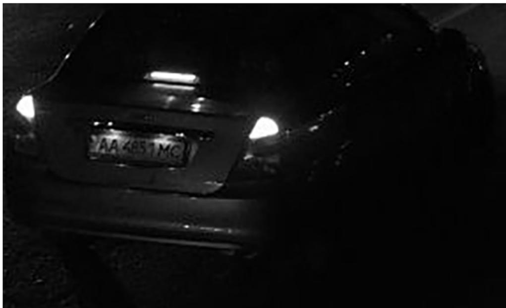
Fig. 16: Insufficient light to recognize license plate
