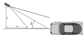
Fig. 11: Horizontal alignment of the camera
