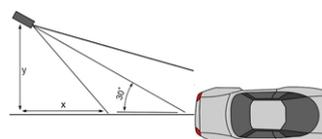
Fig. 11: Horizontal alignment of the camera
