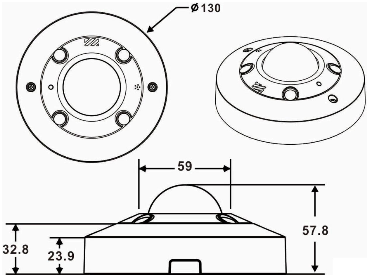
Fig. 1: 12MP Vandal Hemispheric Analytics Indoor Camera: Tutte le misurazioni in mm
