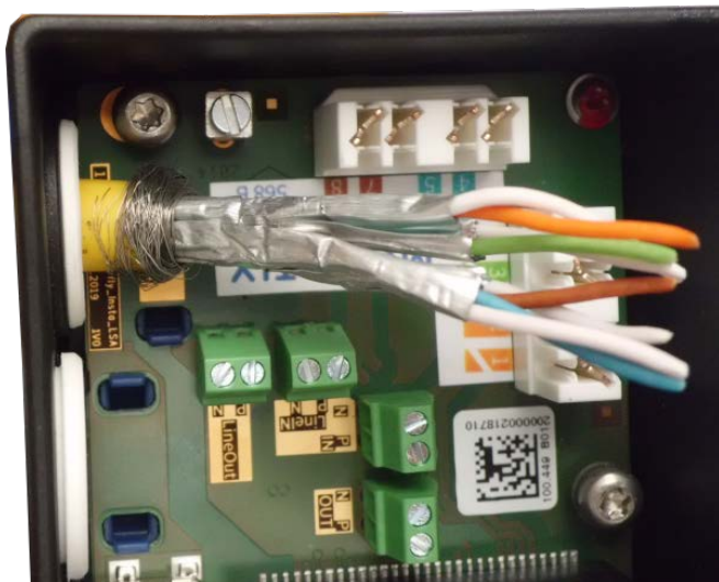
Fig. 23: Network cable inserted, plug properly seated
