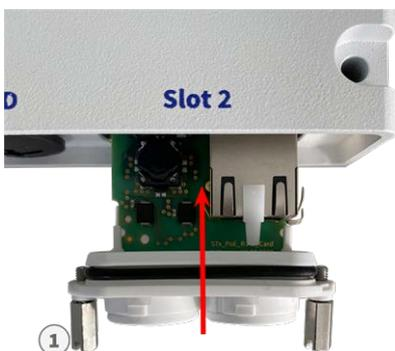
Fig. 6: Collegamento della S74 Network Slide in Board with RJ45 socket
