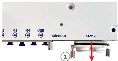
Fig. 5: Remove cover from interface board slot
