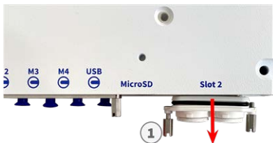
Fig. 9: Remove cover from interface board slot
