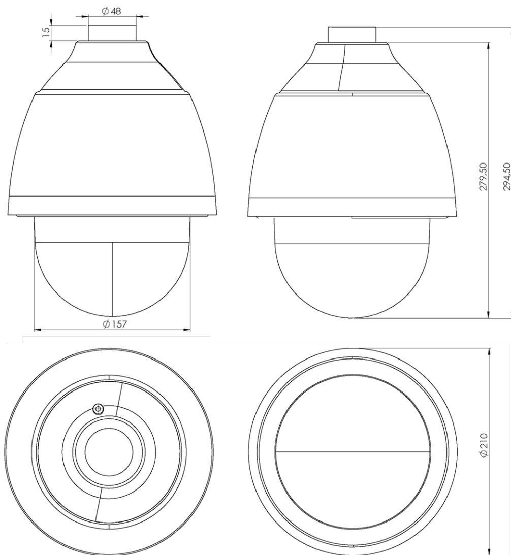
Fig. 1: 2MP Low-Light Video Analytics Speed Dome: Tutte le misurazioni in mm
