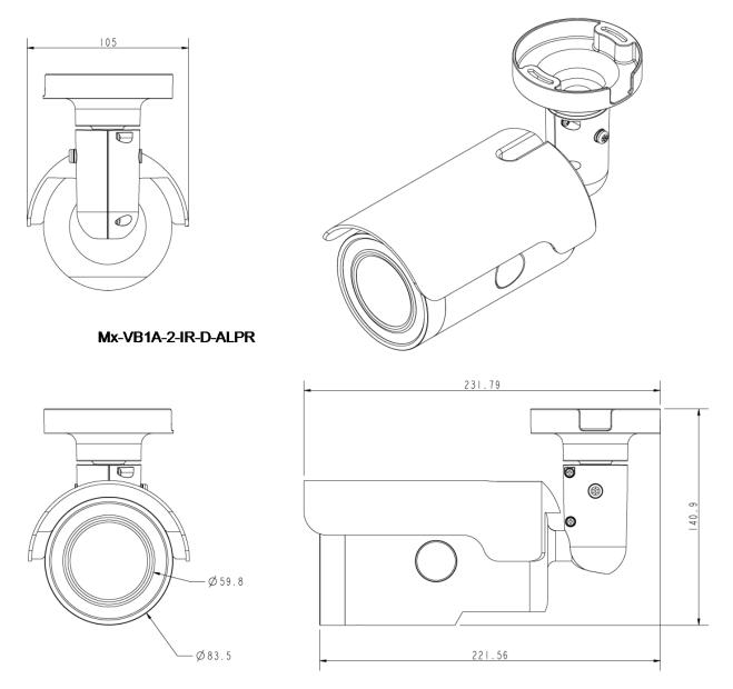
Fig. 2: Mx-VB1A-2-IR-D-ALPR: All measurements in mm
