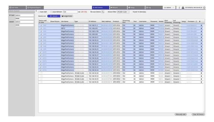
Main Streaming: This streaming is used for Full-Screen view on Live View tab (Default Streaming Source: Stream 1).
