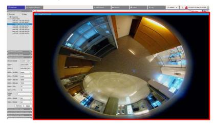
■ **Sub Streaming:** This streaming is used for Multi-Channel view on **Live View** tab (Default Streaming Source: Stream 2).
