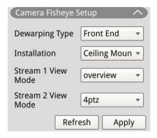
The NVR allows users to adjust dewarping type between Back End dewarping and Front End dewarping depending on the camera's DSP. Select fisheye camera channel and click **Camera Fisheye Setup** on the left to display the settings.
