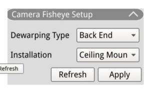
After switching to Back End dewarping mode, icon will appear on the bottom-right corner of the channel grid. includes **Normal View**, **PTZ View**, **360 View**, **Quad View**, **OPR View**, and **103R View**. Select preferred mode and the NVR will automatically dewarp the source
