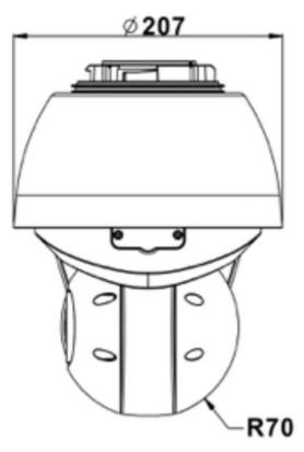
Fig. 1: 5MP IR Video Analytics Speed Dome: All measurements in mm
