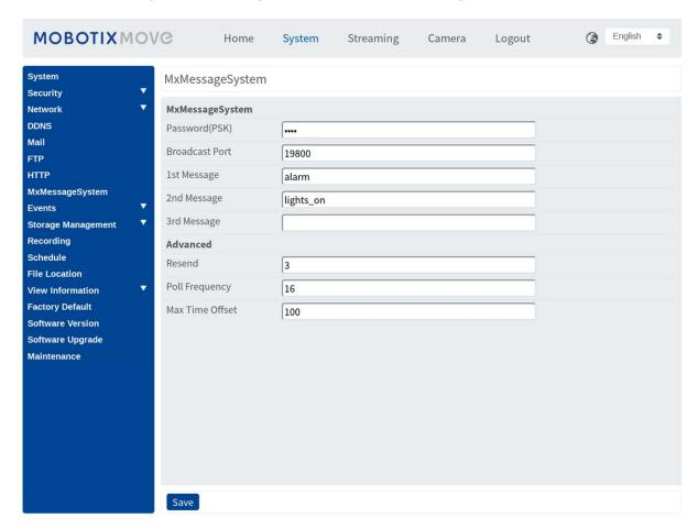
The camera can send notifications via the MxMessageSystem by triggered events.
