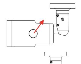
2. Open up the internal cover using a security Torx.
