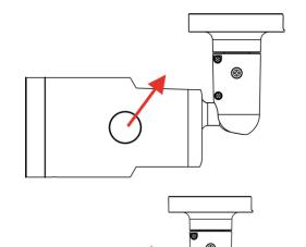
2. Open up the internal cover using a security Torx.
