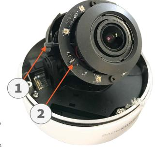
**NOTE!** Take care to properly tighten the focal length lever 1, the focus lever 2, and the screws of the 3-axis gimbal to prevent unwanted changes due to vibration, for example.
