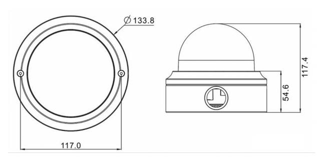
Fig. 1: 2MP Vandal Dome Camera: All measurements in mm
