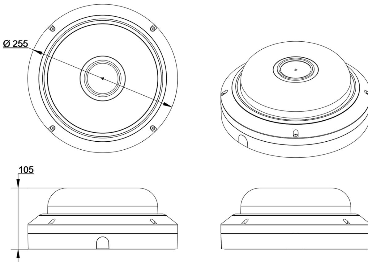
Fig. 1: 20MP Multisensor IR Video Analytics Camera: Tutte le misurazioni in mm
