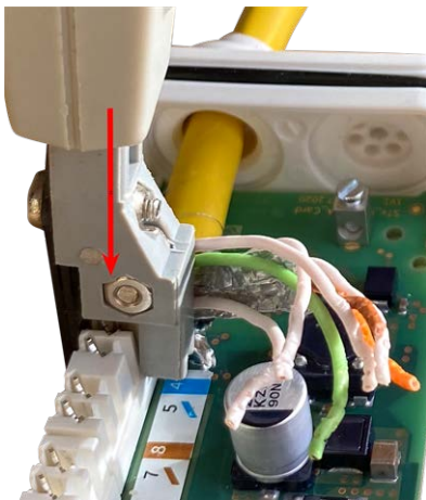
Fig. 13: Network wires connected using LSA+/Krone tool
