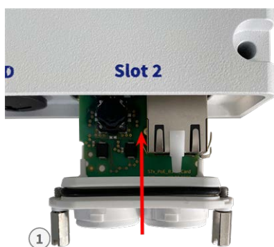
Fig. 6: Connecting the S74 Network Slide in Board with RJ45 socket
