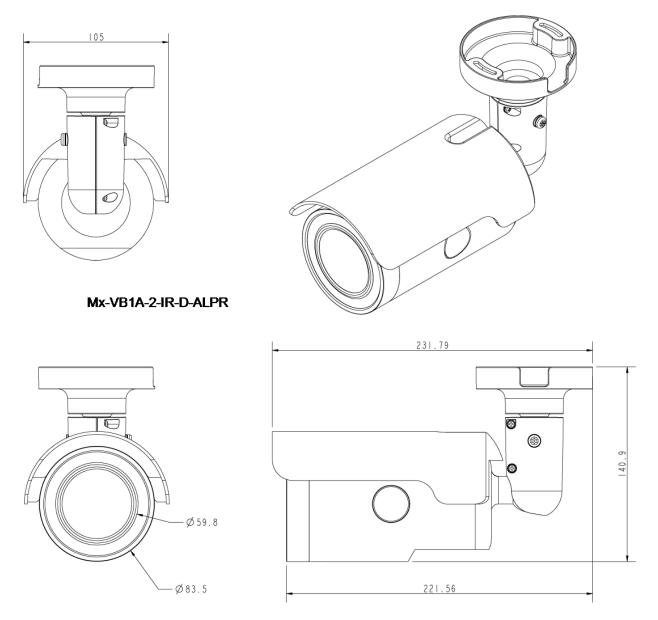
Fig. 2: 2MP Vandal Bullet ALPR Camera: All measurements in mm
