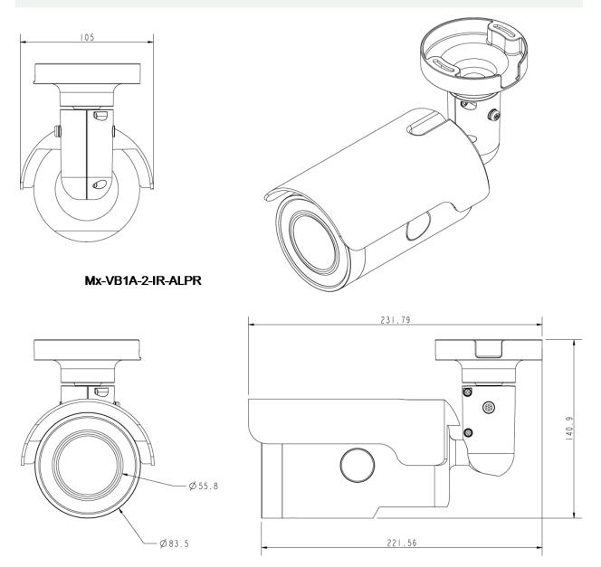
Fig. 1: Mx-VB1A-2-IR-ALPR: All measurements in mm
