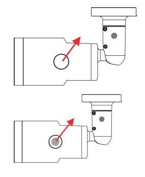
2. Open up the internal cover using a security Torx.
