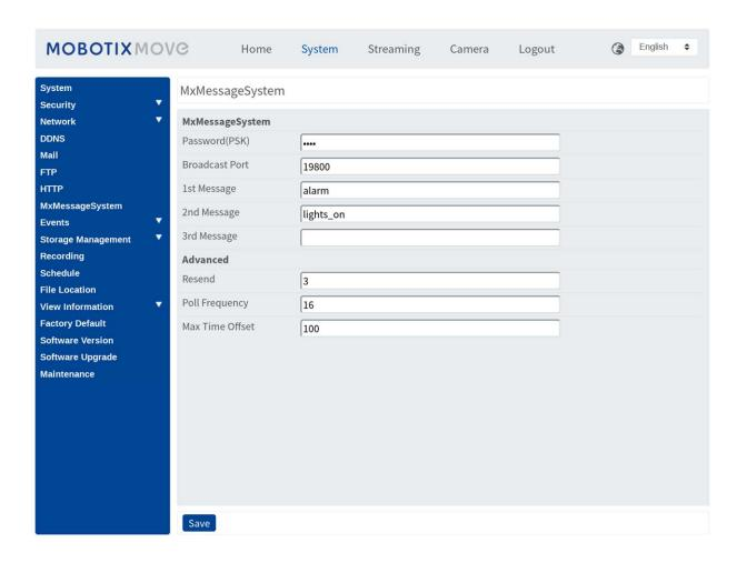
The camera can send notifications via the MxMessageSystem by triggered events.
