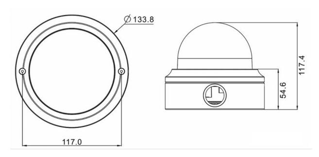
Fig. 1: 5MP Vandal Fixed Dome Analytics Camera: All measurements in mm
