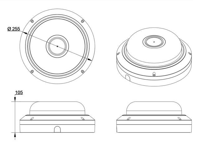
Fig. 1: 20MP Multisensor IR Video Analytics Camera: All measurements in mm
