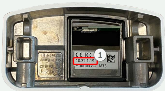
Fig. 2: IP address on the back of the camera housing
