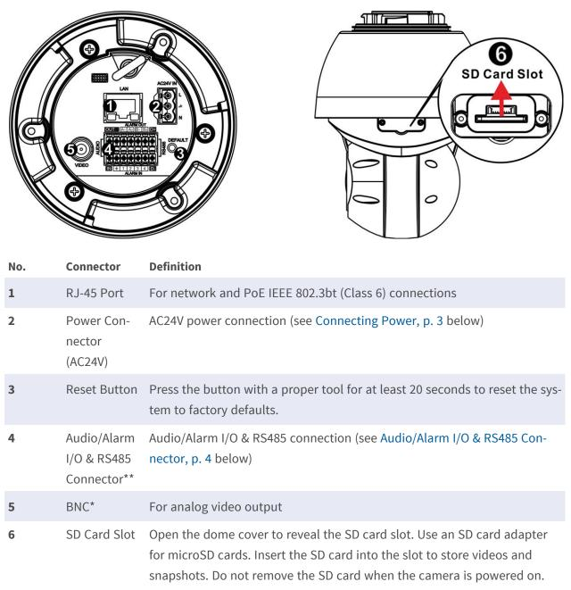
\*Contact the manufacturer for a compatible BNC cable.
