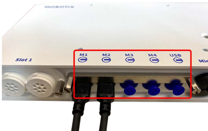
Fig. 22: 4 Module Connector Ports and 1 USB-C interface
