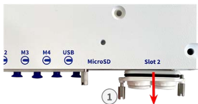
Fig. 5: Remove cover from interface board slot
