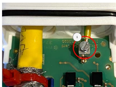
Fig. 15: Ground wire connected to terminal
