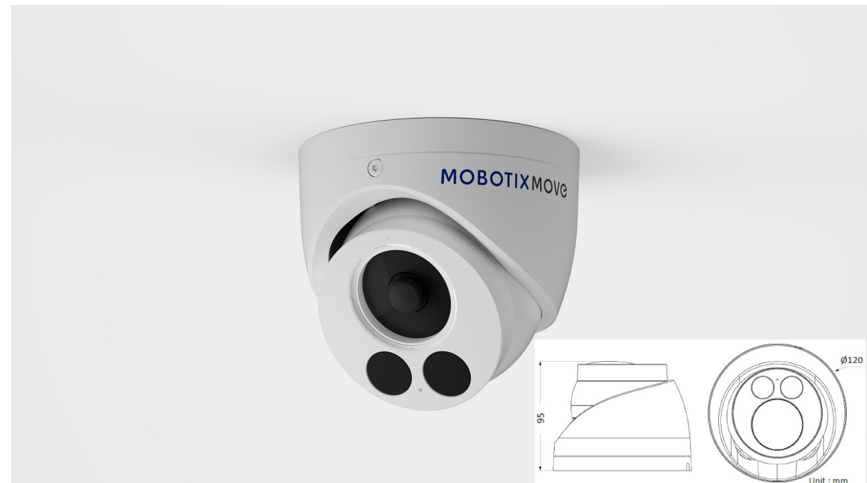
MOVE Turret 2-IR/5-IR with fixed lens, 2MP or 5MP image sensor Field of View (2MP): H: 105°, V: 56°; Field of View (5MP): H: 97°, V: 70.5°
