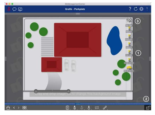
Fig. 45: Changing the camera position on the background image
