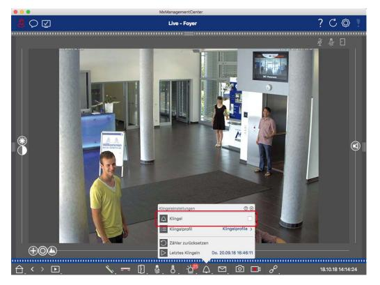
Fig. 53: Turn bell off completely
