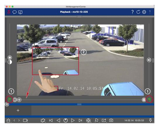
Fig. 147: Adding Clips for Exporting in the Playback View
