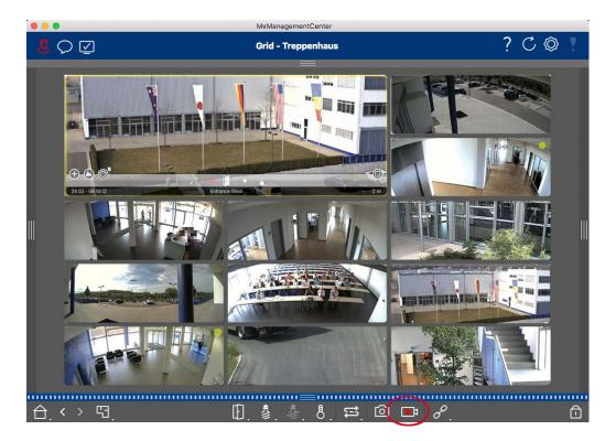
Fig. 121: Manually recording live images
