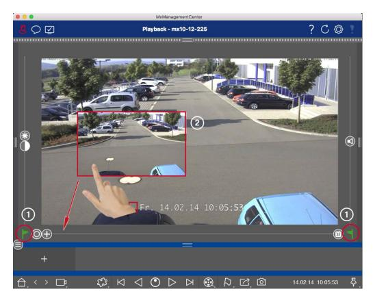
Fig. 4: Adding Clips for Exporting in the Playback View
