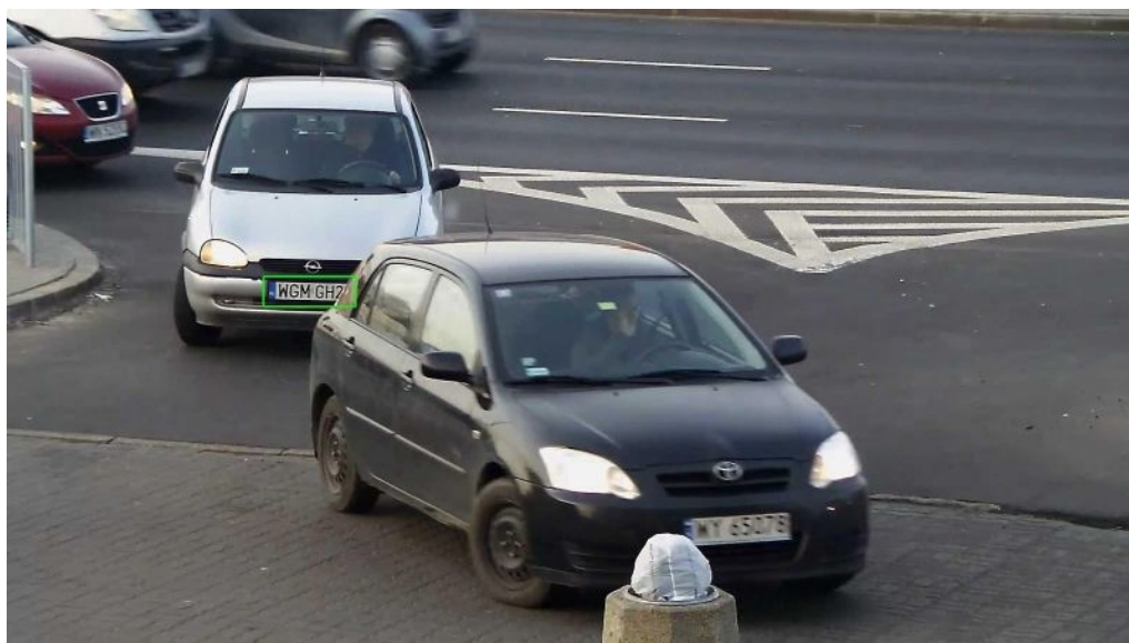
Fig. 11: Insufficient depth of field
