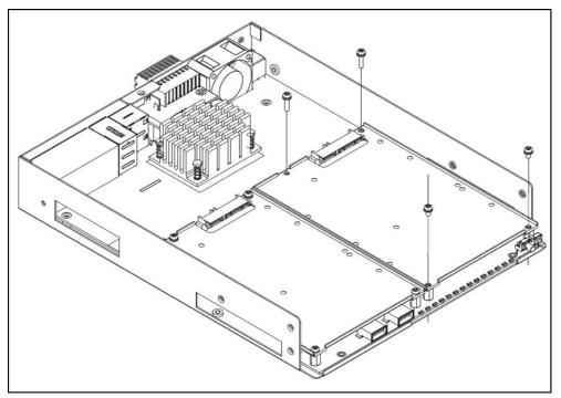
3. Fasten the HDD with the fixing screws delivered with the HDD as shown below.
